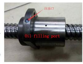
3) Lubrication cycle Observe whether there is an oil film on the surface of the screw during daily inspection. If not, it should be lubricated in time.
