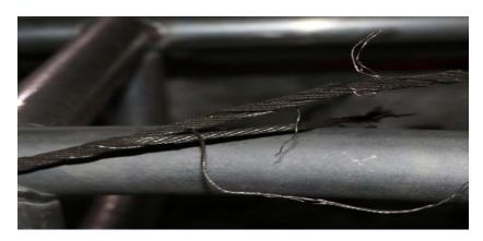
2) Broken wires: When the wire rope has more than six broken wires within the length range of 6 times the diameter or more than 13 broken wires within the length range of 30 times the diameter, the wire should be replaced immediately.
